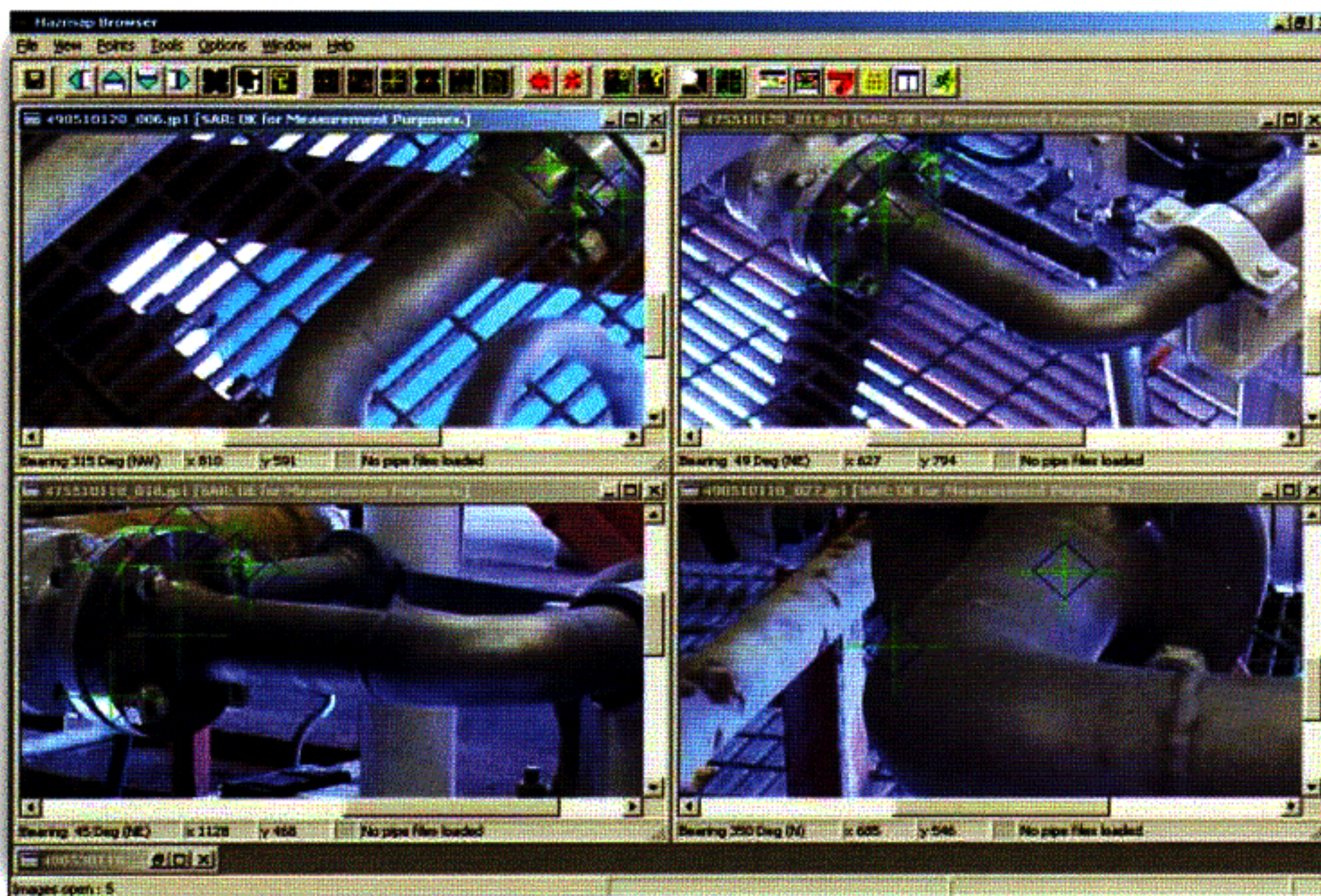
Detailed images of the same location capture from different camera stations allow rapid and precise identification of a point and its co-ordinate to be calculated. (Image courtesy of TWWA)
